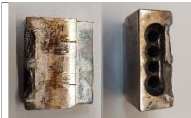
Figura 4. Matrița de reconșionat Figure 4. Mould to be repaired by welding
