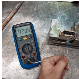
Figura 9. Preîncălzirea piesei de sudat Figure 9. Preheating of the welding part
