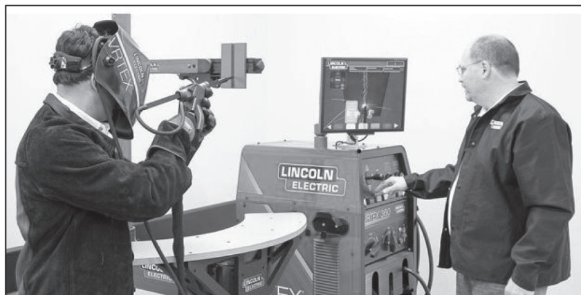
Figura 1. Simulator virtual de sudare Lincoln Electric [13]
