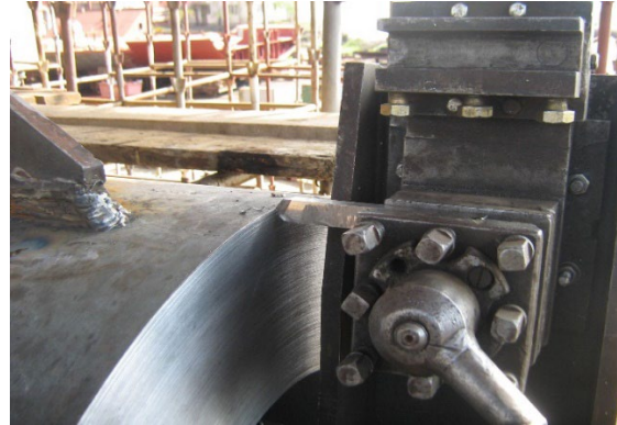
Fig. 8 Prelucrarea zonei frontale prin strunjire Fig. 8 Frontal area machining
