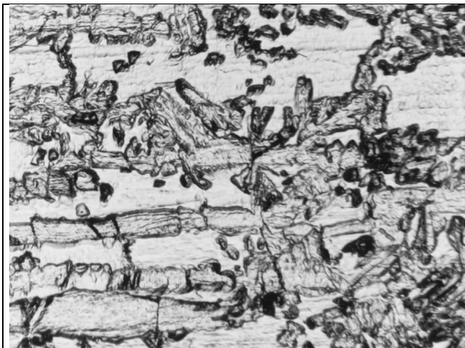
Fig. 5 Microstructura MB, 100x Fig. 5 BM microstructure, 100x
